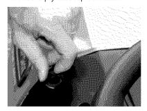
Open tractor hood and ensure that no wires or cables are located at the bottom of the mounting location. If wires or cables are present, temporarily clear the area by securing them safely away from mounting location using a supplied cable tie (J).  Using supplied 9/16" drill bit (DD), drill hole through the dash at the bottom of the mounting location. Use caution not to damage anything in the engine compartment while drilling hole.
